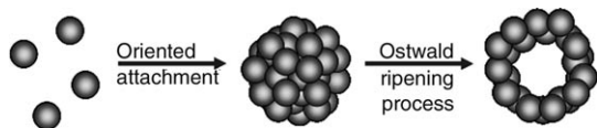
Scheme 1. Schematic presentation of the formation of hierarchical ZnO hollow spheres during the sonochemical process.
